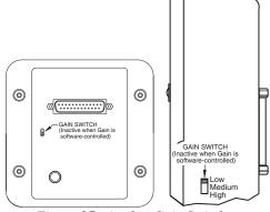
Figure 27. Analog Gain Switch on TE- and LN-cooled Cameras
